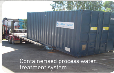
Custom water recycling system for heavy vehicle and equipment washdown
